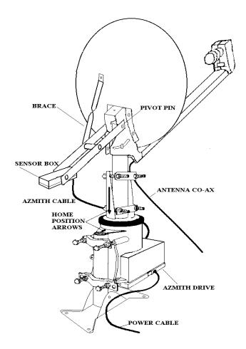
If you have the vertical motor kit assemble it as described below, otherwise retain the plastic tubular spacer and stainless hex bolt in the center holes and attach the brace under one end.
